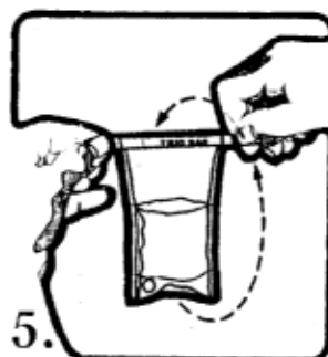
5. Whirl bag 3 complete revolutions. Do not roll tapes down. Leave airspace for mixing in lab.
