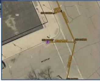
Here's that same inlet in GIS. We see it from above, and can see how it fits into the storm sewer network.
