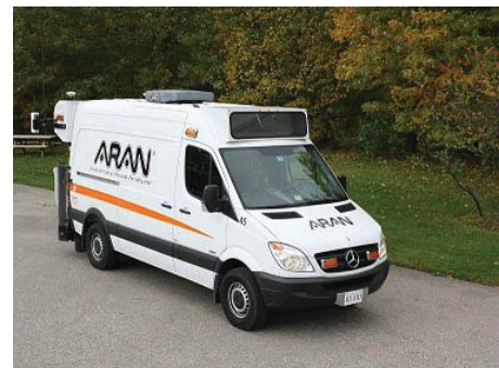
Pavement Scanning Van measures smoothness and cracking
