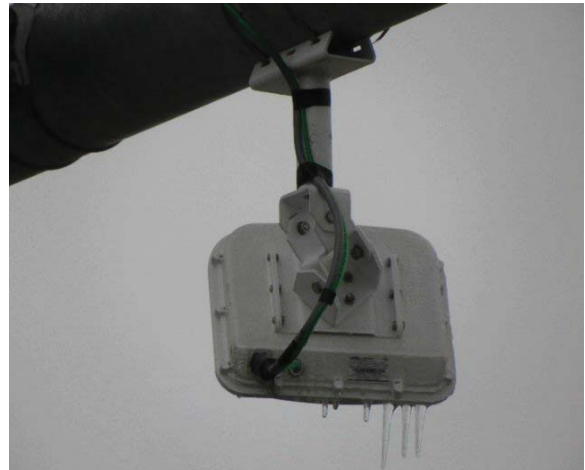
Closeup of a microwave traffic detector
