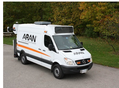
Pavement Scanning Van measures smoothness and cracking
