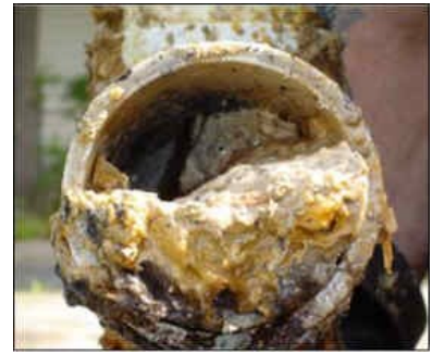
Build up of grease in sanitary sewer pipe
