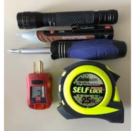
Tools for inspection: flashlight, voltage detector, screwdriver, outlet tester, tape measure
